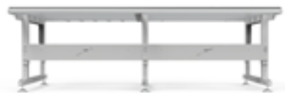
Handling bench Handling bench for sashes and frames Contact surface coated with non-scratch, shockproof material. Prearranged for pneumatic system. Height adjustment. Work table dimensions: 3000 mm x 1300 mm Work table dimensions: 1615 mm x 1300 mm Loading: 120 Kg.
