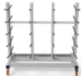
Carr 100 Q Trolley for carriage and storage of profiles in horizontal positions Width: 912mm - Length: 1767mm. Contact surfaces coated with anti scratch and shock-proof plastic material.
