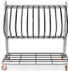
Carr 500 Q Trolley for sashes handling Width: 900mm - Length: 1738mm. Contact surfaces coated with anti scratch and shock-proof plastic material.
