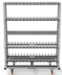
Carr 230 Q / Carr 250 Q Trolley for carriage and storage of profiles in vertical position Carr 230 Q Width: 912mm - Length: 2000mm. Width: 1024mm - Length: 1718mm. Carr 250 Q Width: 1024mm - Length: 1718mm. Width: 1044mm - Length: 2000mm. Contact surfaces coated with anti scratch and shock-proof plastic material.
